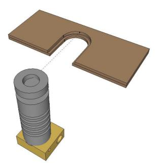
Mount these on to the top side of the X carriage. The top part of the peek barrel should jut above the MDF plate and fit in to a circular hole in the extruder block.
