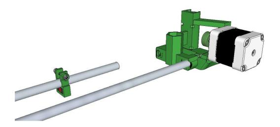
Then slide the X carriage on to the two rods carefully engaging each rod in to the linear bearings of the carriage. The belt clamp part of the carriage must be on the same side as the motor to ensure the belt will fit properly.
