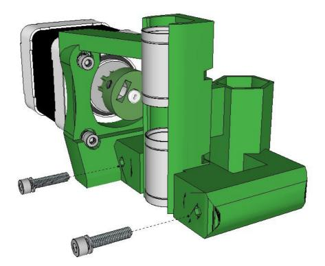
The final preparation is to assemble the X axis endstop. Insert a wired microswitch into the slot as shown and insert a m3x20 cap screw, washer and nut. Do not tighten the nut yet. Note, ensure the middle terminal and the one at the same end as the red button are wired (so the switch will make rather than break contact when the red button is pressed) and have heat shrink insulation.
