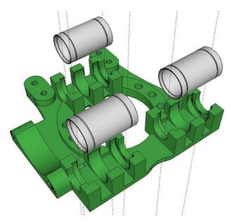
Then carefully press down gently but firmly with pressure applied evenly along the bearing length until it clips in to place. Repeat for the other two bearings making sure all bearings are fully and properly seated in the clips.
