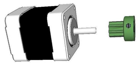
Attach the stepper motor to the X motor bracket using three M3x10 cap screws and possibly washers (these may not fit on your bracket depending on how it was printed).
