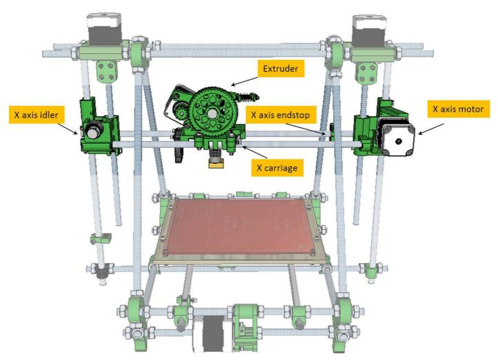
This section describes the construction of each of these in turn together with their overall assembly in to the X axis as shown below;
