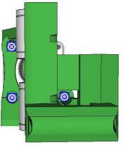
Note how the three cap screw heads are accessed, highlighted in the diagram on the left.
