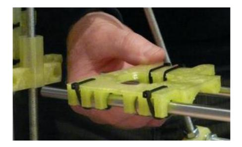
Next, attach the belt clamps as shown using M3x20 cap screws and washers for the single clamp and M3x30 cap screws and washers for the double clamp. All four bolts are then secured using nyloc nuts.
