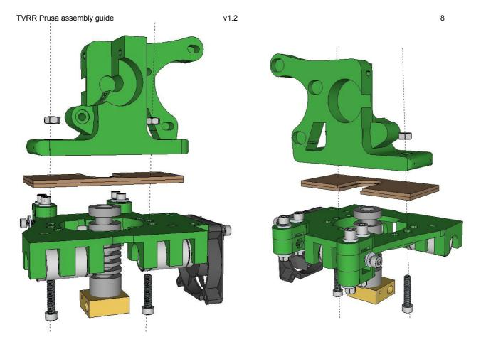
If the MDF to x-carriage mounting is a bit loose this can be addressed by placing 2 or so M8 washers in the extruder block well to close the gap with the top of the PEEK barrel.
