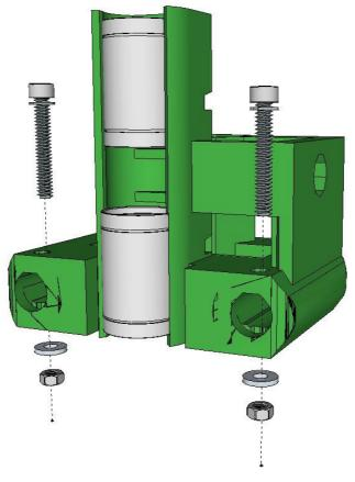
Thread the M8x60 hex head bolt into a washer, two 608 bearings and another washer. Insert this loaded bolt into the out hole of the idler bracket and secure using a washer and nut.Note: the 13mm spanner will not fit into the gap so another method will be needed to prevent the nut turning. (The author used one jaw of a pair of pliers loosely inserted in the gap between nut and bracket.)
