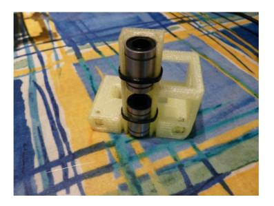
Insert the two M3x20 cap screws with washers and nyloc nuts in to the holes near one end of the rod slots. These cap screws prevent the bracket moving along the smooth rods and provide a firm and even "wall" for the rods to be tensioned against.
