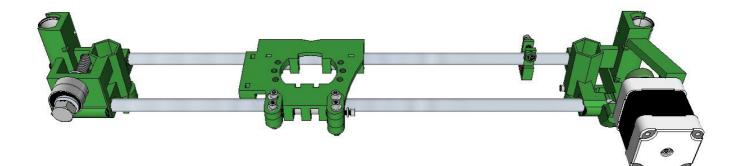
The first step is to test fit and ease various parts to make sure that they will fit properly when assembling the X axis on the machine. You need to do this now because it is easier than when the X axis is already mounted and you won't disturb the overall structure and alignment of the machine.
