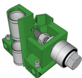
Start by locating and carefully pressing down with pressure applied evenly along the bearing length until it clips in to place.
