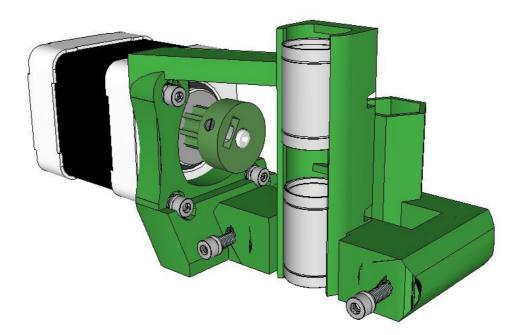
Prepare a pulley by inserting an M3 nut into the captive slot and the grub screw.
