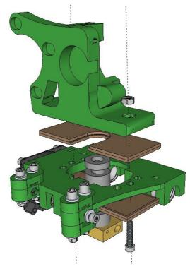
**Remove all the bits you have test fit on to the X carriage.** You will now assemble the X carriage proper.
